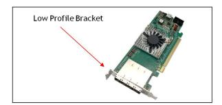
For low profile case applications, change the mounting bracket to the low profile bracket. You can order a low profile bracket by contacting our Sales Support. Replacing the "High Profile Bracket" with "Low Profile Bracket" is done by removing the screws that hold the card to the bracket. Detach the standard bracket from the card, and place the low profile bracket and secure it. Use proper ESD procedures when completing this action.
