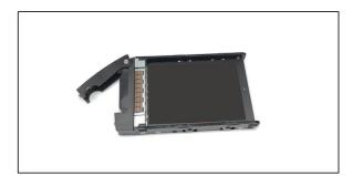
Insert the hard drive and drive carrier into its bay vertically, keeping the carrier oriented so that the release button is on the top. When the carrier reaches the rear of the bay, the release handle will retract.
