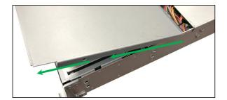
After removing the front top cover, next is to remove the back-end top cover. Lift the back-end top cover and slide it out.
