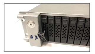
Grasp the handle and gently pull the drive tray out of the chassis.
