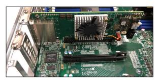
Then secure the card to the slot with a mounting screw.
