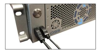
Plug-in the VGA (external display) and Ethernet cables.
