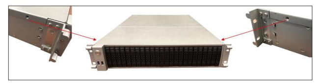
Remove the screw located on the top-end of the cover, see photo below
