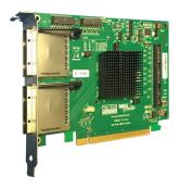
PCIe x8 Gen 3 dual-port, switch-based cable adapter with DMA controller and optional NT ports. The cable adapter operates in I/O expansion or with a DIP switch setting change.
