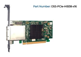
PCIe x16 Gen 3 switch-based cable adapter with an NT port and a DMA controller. The cable adapter operates in I/O expansion or networking mode with a DIP switch setting change.
