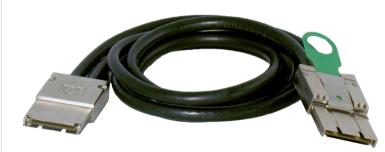
PCIe x8 expansion cable with PCIe connectors. With crossover cabling, the connectors on either end of the PCIe x8 cable are identical. Each connector is equipped with a retractor allowing the connector to be locked into place.
