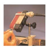
A shop vac may be attached to the plastic tube to remove dust particles. To keep the pieces you are sanding from being sucked into the vacuum put a piece of plastic screening, available from hardware stores, over the end of the tube, before attaching the hose. Light pressure on the belt while sanding, will give the quickest results and longer belt life.
