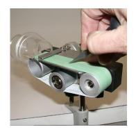
The Ikohe Belt Sander can be worked at any position that makes sense for your desired task, including on the end, on the flat plate on the top or In between the wheels on the back. The Ikohe Belt Sander is ideal for sprue removal, bench work, graver/chisel sharpening; tool making modification and more.
