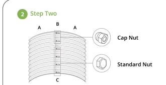
Cap nuts are used for top two rows, standard nuts are used for lower 4 rows. Assemble all curved panels: initially attach all bolts, washers and nuts loosely, and then tighten up using the wrench tool (as supplied) with a screwdriver/cordless drill.
