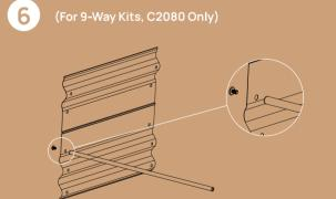
Bracing rods are used to reinforce the strength of long raised beds. Only the 2ft x 8ft configuration requires a 2ft wide bracing rod. Install the rod between two parallel bolt holes. Attach the bolt, panel and rod loosely, and ensure the rod is connected through the third bolt hole from the top. Finally, fasten it tightly with a screwdriver to reinforce your raised bed.
