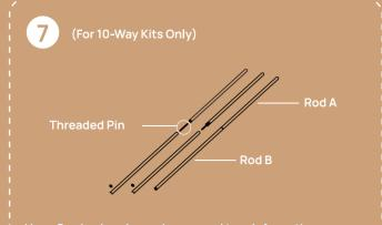
Vego Garden bracing rods are used to reinforce the strength of large raised beds. For C4080, C2580, C2595, C4065, and C2575 configurations, we recommend the use of bracing rods. For 2.5ft wide raised beds, use Rod A only; and for 4ft wide raised beds, use the threaded pin provided to connect Rod A and B.
