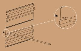
Install the bracing rod between two parallel bolt holes. Attach the bolt, panel and rod loosely, and ensure the rod is connected through the third bolt hole from the top. Finally, fasten it securely with a screwdriver. Now, your garden bed installation is complete! Happy gardening!
