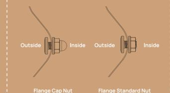
After the straight panels are assembled, attach corner panels to straight panels via the same method. Make sure the corner panels are attached on the outside of the straight panels.
