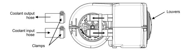
Inspect for coolant leaks
