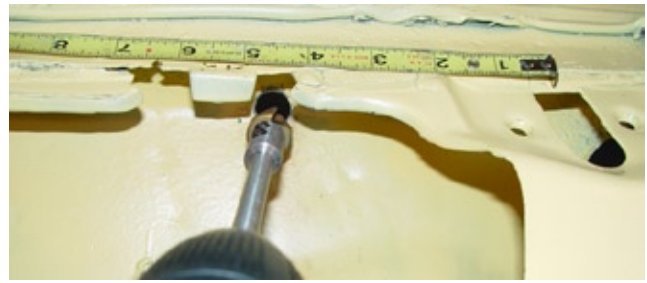
Photo 2. Drill the wiring pass through hole 4" to 6" (not more than 6") inboard of the middle of the driver side pivot shaft opening,
