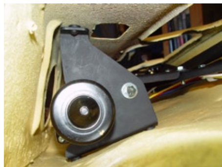
Photo 18a. Insert the Motor Brace into the air box. The crescent shape in the brace fits onto the body of the motor itself. Raise the Motor Plate with one hand and with the other orient the 1/4" hole on the middle of the Motor Brace with the 1/4" threaded boss on the Motor Plate. Secure with a 1/4-28 bolt and flat washer.
