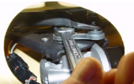
Photo 15. Put the Drive Arm onto the Motor Spindle. Looking through the small rectangular hole on top of the cowl air box. Rotate the Drive Arm counter clockwise (CCW) on the Motor Spindle until the "C" shaped detail on the Drive Arm comes to rest over an empty, 1/4" hole in the Motor Plate. . Pass a long 1/4" bolt or the shaft of a phillips screwdriver through the "C" detail of the Drive Arm and into the 1/4" hole on the Motor Plate and tighten Spindle Nut.
