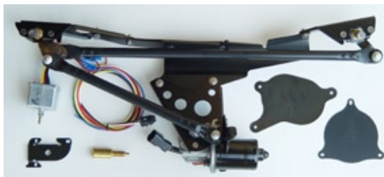
Photo 00 shows the system as it will look assembled in the air box. Optional variable delay switch and 68-69 and 67 coverplates shown. 69 switch adapter shown.
