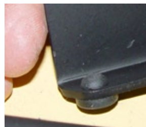
Photo 18. Put three rubber bumpers into the Motor Brace flange holes.
