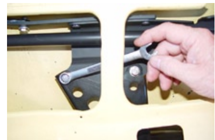
Photo 12. Use two 1/4" bolts and flat washers to secure it. Tighten these bolts.
