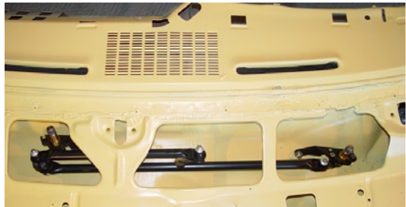
Photo 4. The entire Drive Unit Assembly should end up with the tips of the Pivot Shafts pointing in an upward and aft position. In this photo the Drive Unit Assembly is resting on the bottom of the air box with the Pivot Shafts to the left of their respective pivot shaft openings in the cowl.
