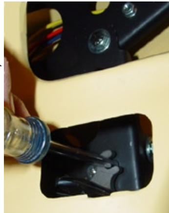
Photo 15. Put the Drive Arm onto the Motor Spindle. Looking through the small rectangular hole on top of the cowl air box. Rotate the Drive Arm counter clockwise (CCW) on the Motor Spindle until the "C" shaped detail on the Drive Arm comes to rest over an empty, 1/4" hole in the Motor Plate. . Pass a long 1/4" bolt or the shaft of a phillips screwdriver through the "C" detail of the Drive Arm and into the 1/4" hole on the Motor Plate and tighten Spindle Nut.
