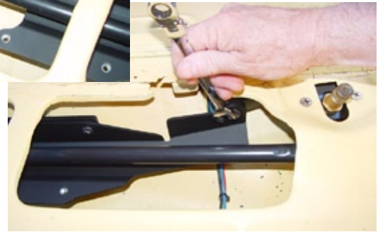
Photo 10. Tighten the left Pivot Shaft Assembly bolts. Then tighten the 4, Countersunk, 1/4" phillips head bolts in the cowl.
