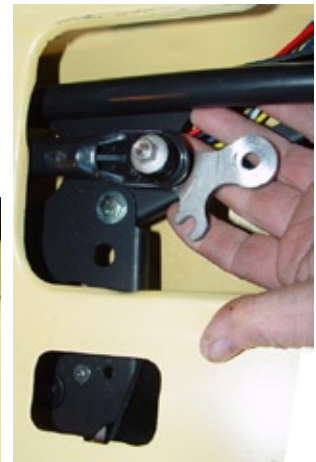
Photo 14. Position the open hole in the drive arm over the Motor Spindle. Lower the Drive arm onto the Motor Spindle.
