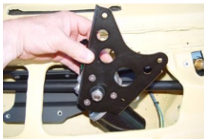
Photo 11. Insert the Motor Plate into the air box. Orient the two 1/4" holes with the threaded bosses near the center of the Bridge.
