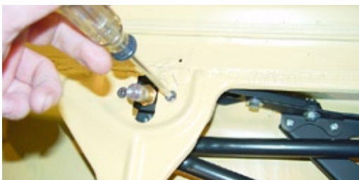
Photo 7. Secure each side with two 1/4" countersunk screws but do not tighten yet. Leave them about one turn shy of tight.
