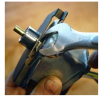
Photo 23. You can attach the Switch to the Switch Adapter Plate before installing it in the dash.
