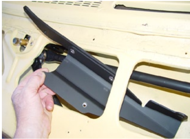
Photo 8, Insert the Bridge (B) into the airbox.
