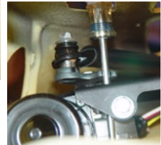
Photo 16. is taken inside the cowl air box looking from the driver side towards the passenger side. The original motor hole is to the left
