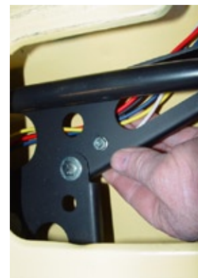
Photo 13. Route the harness wires under the Bridge.
