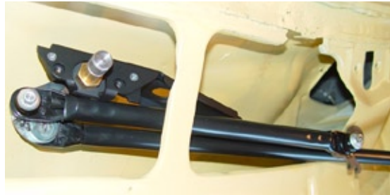
Photo 2. Drill the wiring pass through hole 4" to 6" (not more than 6") inboard of the middle of the driver side pivot shaft opening,
