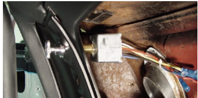
Photo 21. This photo shows the 1967-68 Delay Switch installed in the dash. The delay switch for this application is supplied with a (brass) 3 piece extension to clear the rear of the dash.
