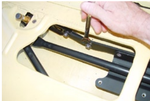
Photo 10. Tighten the left Pivot Shaft Assembly bolts. Then tighten the 4, Countersunk, 1/4" phillips head bolts in the cowl.
