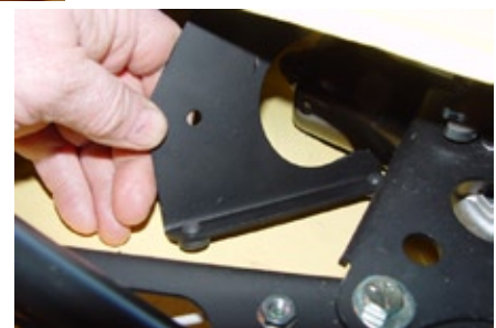
Photo 18a. Insert the Motor Brace into the air box. The crescent shape in the brace fits onto the body of the motor itself. Raise the Motor Plate with one hand and with the other orient the 1/4" hole on the middle of the Motor Brace with the 1/4" threaded boss on the Motor Plate. Secure with a 1/4-28 bolt and flat washer.
