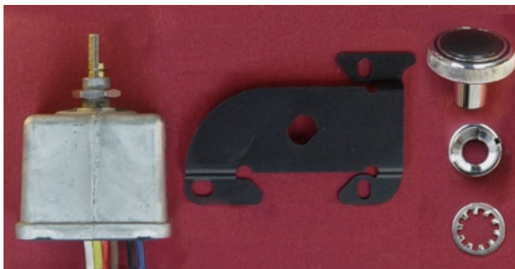
Photo 24. This photo shows the later 1969 -74 Delay Switch and installation hardware. Your switch may look different, depending on the year of your car and type of switch.
