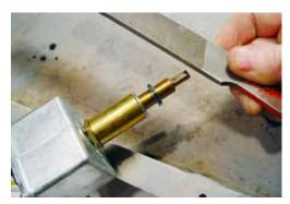
(Fig 09-03) File a flat spot in the shaft at the 6 o'clock position for the switch knob's set screw.
