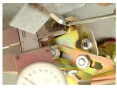
(Fig 08-02) Adjusting the parked position of the Pivot Shaft is done in the same way as the Passenger side.
