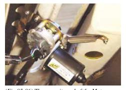
(Fig 05-06) The opposite end of the Motor Brace goes up against the underside of the firewall where the left side of the old (OEM) wiper motor was attached. Attach the Brace using a 10-32x3/4" phillips, washer, and nut. This same fastener holds one side of the new Cover Plate.
