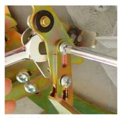
(Fig 07-05) On the driver side loosten the two phillips head screws, extend or retract the Link Tip as needed clear both the defroster duct and the brake pedal/clutch pedal bracket. Retighten the screws.
