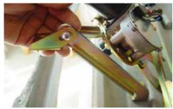
(Fig 09-02) Attach the other end of the Windshield Brace to the Windshield Brace Mounting Bracket mounted under the Cover Plate.
