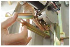
(Fig 09-01) Attach the Windshield Brace on the middle right hand windshield attachment bolts.
