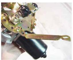
(Fig 05-03) Attach the Motor Brace.
