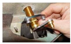
(Fig 06-02) Place the two shotted holes onto the 10-24 studs.
