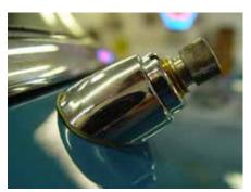
(Fig 06-05) Add the passenger side Crome Ecutcheon and chrome Escutcheon Nut.
