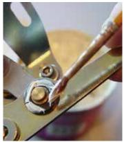
(Fig 07-01) Put a dab of thick axle grease on the exposed side of the plastic bushing before placing the very thin flat washer onto the exposed brass pivot pin, sticking it to the grease on the plastic bushing.
