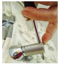
(Fig 06-06) When you are satisfied with the fit of the Pivot Shaft and chrome escutcheon fit on the outside of the car, tighten all interior screws before installing the chrome escutcheon nut with the aluminum Escutcheon Wrench supplied in the kit. Overtightening can damage the fiberglass.
