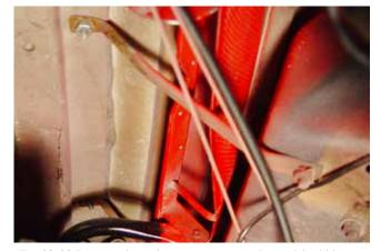
(Fig 02-03 Remove the right, or passenger side windshield brace rod.
