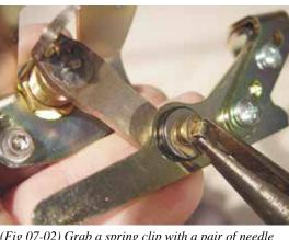
(Fig 07-02) Grab a spring clip with a pair of needle nose pliers. Slip the spring clip over the brass pivot pin, press towards the thin washer/plastic bushing and secure the clip into the groove in the shaft.
