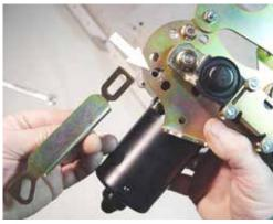
(Fig 05-02) Use a 10mm wrench to remove the motor mounting screw as shown
