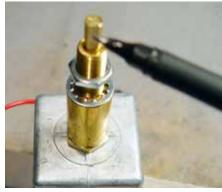
(Fig 09-04) File enough to allow the set screw to securely clamp the knob to the shaft.
