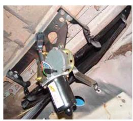
(Fig 05-05) Place the Main Drive Unit up against the underside of the cowl, between the cowl vent hinge brackets. Use four 1/4-20x3/8" hex bolts and 1/4" flat washers to hold the Main Drive Unit and cowl vent brackets in place.
