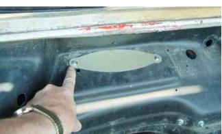
(Fig 08-05) The Cover Plate goes where the old motor was mounted. (53-57 Cover Plate shown.)
