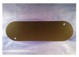
(Fig 08-03) A Cover Plate is supplied to cover the hole left in the firewall from the old wiper motor. 58-62 shown
