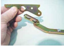
(Fig 03-05) Sandwich the Link Tip between the Link and the Link End Stiffener.
