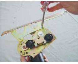
(Fig 05-01) Using two 10-32x3/8 screws, nuts and washers, attatch the motor to the motor mount bracket.
