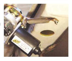
(Fig 08-04) The Motor Brace was attached to the cowl so the wiper unit could be installed and adjusted. The Windshield Brace Mounting Bracket will be added at that location. (53-57 shown)
