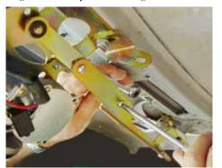
(Fig 07-03) Passenger side Link length adjustment. Loosen the two phillips head screws that attach the long and short Link halves. Slide them apart or together to adjust the length.
