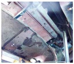
(Fig 05-04) Remove 4 1/4-20 hex bolts holding the cowl vent hinge brackets to the under side of the cowl.
