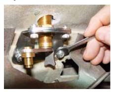
(Fig 06-03) Secure the Pivot Shaft Bracket to the body.
