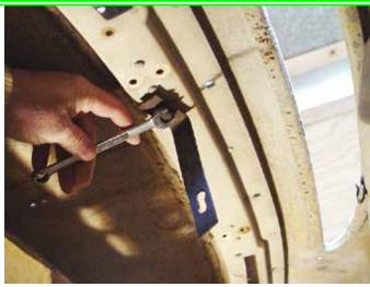
(Fig 02-01) Remove the radio support.
