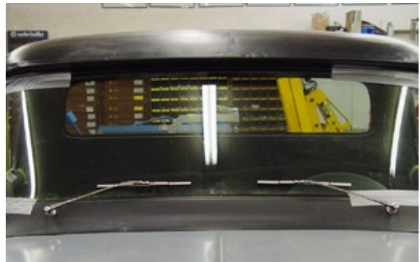
Photo 22. This photo shows the Wiper Arms and Blades installed on the truck.
