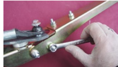
Photo 6. Use the 1/4" flat washers and hex nuts.
