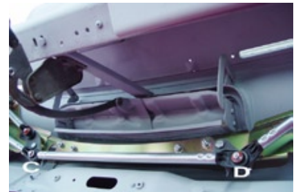
Photo 15. Replace the cupped lock nuts and tighten them with a 3/8" 12 point box end wrench per the note.
