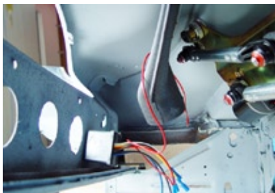
Photo 17. Insert the switch through the backside of the hole on the dash.
