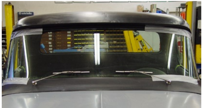
This photo shows the Wiper Arms and Blades installed on the truck.
