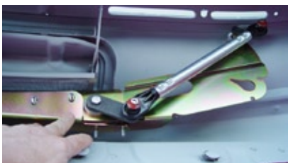
Photo 10. On the passenger side, insert the Pivot Shaft of the Follower Unit into the wiper hole. As you do so, join the 4 carriage bolts in the Follower Assembly to the Bridge Spanner.
