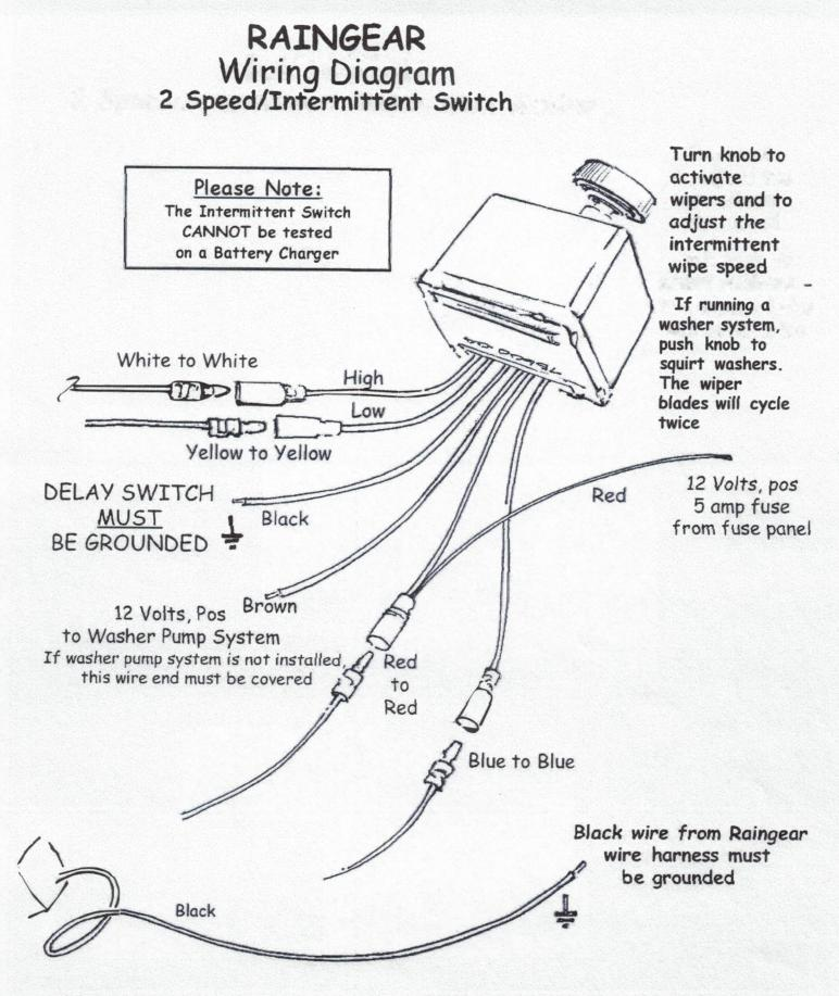
**NOTE:** The colors of the wires from the wiper motor and the colors of the wires on the harness do not match. This is correct.
