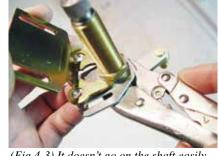
(Fig 4-3) It doesn't go on the shaft easily. You might find it easier to gently hold the Pivot Shaft with vice grips.
