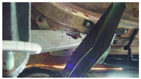
(Fig 8-3) This shows an early version of the Pivot Shaft Mounting Plate installed above the metal substructure.
