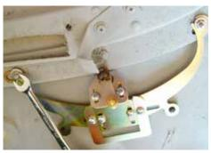
(Fig 9-2) Place #12-24 hex nuts and 1/4" flat washers on the windshield retaining studs and tighten them.
