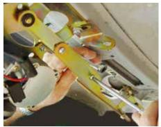
(Fig 11-3) Passenger side Link length adjustment. Loosen the two phillips head screws that attach the long and short Link halves. Slide them apart or together to adjust the length.
