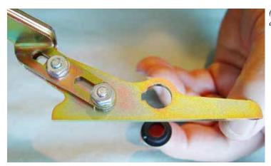
(Fig 6-4) Push the Plastic Bushing into the keyed hole as far as it will go.
