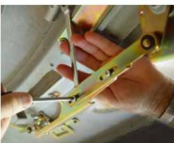
(Fig 12-1) Driver side Link length adjustment.
