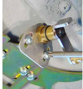
(Fig 10-2) The other primary, up and down, adjustment is by loosening the two phillips head screws of the aluminum Pivot Shaft Holding Plate so it can be adjusted.
