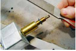
(fig 13-3) File a flat spot in the shaft at the 6 o'clock position for the switch knob's set screw.
