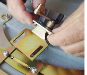
(Fig 8-1) This is the passenger side looking aft. The fiberglass cowl has been removed. This Corvette has the metal substructure that requires separating the Pivot Shaft Orientation Brackets from the Pivot Shaft Mounting Plates and "U" Guides to install the Pivot Shaft Mounting Plates and "U" Guides between the metal substructure and fiberglass cowl.
