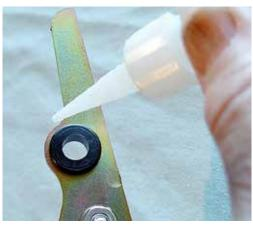
(Fig 6-6) Use a very thin bead of super glue to secure the Plastic Ring to the Plastic Bushing.
