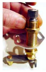
(Fig 4-1) Add the flat aluminum Pivot Shaft Holding Plate down to the first hex nut and install a second 5/8-24 hex nut.
