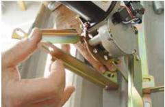
(Fig 13-1) Attach the Windshield Brace on the middle right hand windshield attachment bolts.
