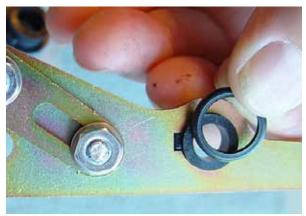
(Fig 6-5) The Plastic Bushings that fit into the keyed holes in the Link Tips have a plastic ring that fits on the side that extends through the keyed hole.
