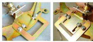
(Fig 4-6 & 4-7) Using the 10-32x3/8" phillips head screws and washers, attach the Pivot Shaft Orientation Bracket to the Pivot Shaft Mounting Plate.
