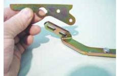
(Fig 5-5) Sandwich the Link Tip between the Link and the Link End Stiffener.
