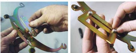
(Fig 3-6 & 3-7) On the opposite side of the pivot shaft Mounting Plate, the 4 nut backing strip is used to attach the "U" Guide to the Mounting Plate.
