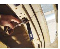
(Fig 2-2) Remove the radio support.
