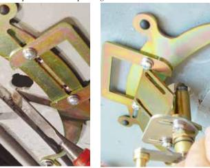
(Fig 9-3) Some Corvettes need the excess glue, aft of the pivot shaft, removed so the new pivot shaft will fit properly.
