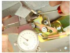
(Fig 12-2) Adjusting the parked position of the Pivot Shaft is done in the same way as the Passenger side.
