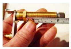
(Fig 3-8) Run a 5/8-24 hex nut down the threads of each pivot shaft about 2 3/8"
