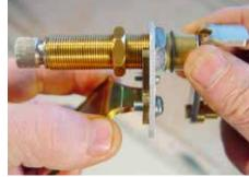
(Fig 10-3) Loosen the 5/8-24 hex nut closest to the tip and rotate it toward the tip by the distance you want to pull the tip closer to the cowl.
