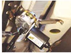
(Fig 7-6) The opposite end of the Motor Brace goes up against the underside of the firewall where the left side of the old (OEM) wiper motor was attached. Attach the Brace using a 10-32x3/4" phillips, washer, and nut. This same fastener holds one side of the new Cover Plate.
