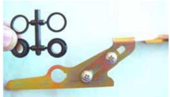
(Fig 6-1) The Plastic Bushings that fit into the keyed holes in the Link Tips & opposite Link ends.
