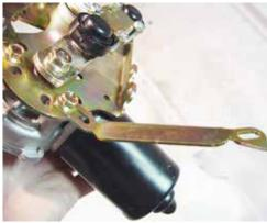
(Fig 7-3) Attach the Motor Brace.
