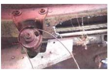
(Fig 2-3) On 1956-57, remove the spool and cable assembly.
