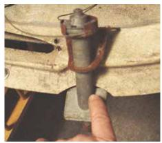
(Fig 2-4) Remove the pivot shafts.
