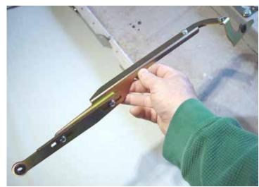
(Fig 5-3) The complete passenger side Link assembly with the longer and shorter links attached.
