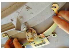
(Fig 9-1) You can install the Pivot Shaft Mounting Assembly as a single unit, including the Pivot Shaft, on cars without the metal sub structure. This photo shows the passenger's side.
