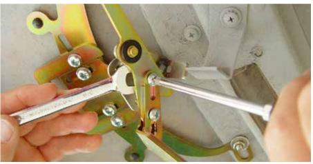
(Fig 11-5) On the driver side loosten the two phillips head screws, extend or retract the Link Tip as needed clear both the defroster duct and the brake pedal/clutch pedal bracket. Retighten the screws.
