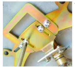
this, loosen the four phillips head screws holding the Pivot Shaft Orientation Bracket and "U" guide to the Pivot Shaft Mounting Plate. (Fig 9-5) The outside two secure the "U" guide and provide side to side adjustment. Retighten the outside two once the shaft is centered from side to side. The inside two provide up to down centering within the hole in the cowl. It also helps provide in and out adjustment of the Pivot Shaft tip. Center the Pivot Shaft and tighten the inside two screws.
