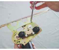
(Fig 7-1) Using two 10-32x3/8 screws, nuts and washers, attatch the motor to the motor mount bracket.
