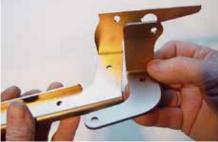
(Fig 5-1) Attaching the Corner Stiffener to the passenger side Link.
