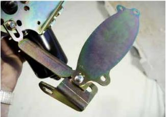
(Fig 12-6) This photo illustrates how the Motor Brace, Windshield Brace Mounting Bracket and Cover Plate share the same mounting point.
