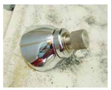
(Fig 10-5 & 10-6) When you are satisfied with the fit of the Pivot Shaft and chrome escutcheon fit on the outside of the car, tighten all interior screws before installing the chrome escutcheon nut with the aluminum Escutcheon Wrench supplied in the kit. Overtightening can damage the fiberglass.
