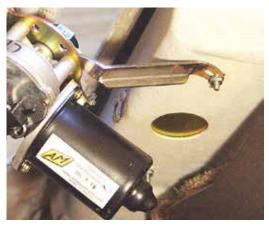
(Fig 12-5) The Cover Plate goes where the old motor was mounted.
