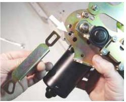
(Fig 7-2) Use a 10mm wrench to remove the motor mounting screw as shown
