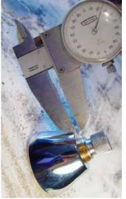
(Fig 10-1) With the chrome escutcheon placed onto the Pivot Shaft and resting on the body, 1/8" to 3/16" of the brass threads of the Pivot Shaft should be showing.
