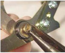
(Fig 11-02) Grab a spring clip with a pair of needle nose pliers. Slip the spring clip over the brass pivot pin, press towards the thin washer/plastic bushing and secure the clip into the groove in the shaft.
