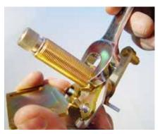
(Fig 4-5) Run the hex nut down to the Pivot Shaft Orientation Bracket about finger tight.
