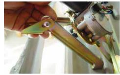
(Fig 13-2) Attach the other end of the to the Windshield Brace to the Windshield Brace Mounting Bracket mounted under the Cover Plate.
