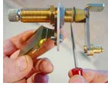
(Fig 10-4) Slide the Pivot Shaft Orientation Bracket and Pivot Shaft Holding Plate up against that 5/8-24 hex nut. Tighten the other 5/8-24 hex nut up against the Pivot Shaft Holding Plate. The pointer shows the distance the tip of the Pivot Shaft will be moved closer to the cowl.
