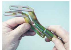
(Fig 5-4) Match the outer end of the longer Link to the Link End Stiffener.
