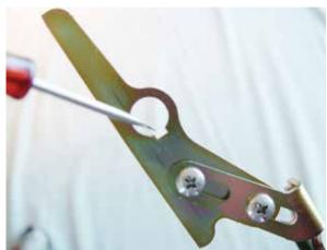
(Fig 6-3) This shows the keyed hole in the Link Tip.
