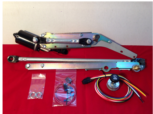
Fig 1: This is the kit as shipped. It is broken down for shipment and will need to be reassembled per the instructions on the following page.
