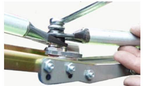
Fig 5: Right - Do not tighten the cup nut too much. Pull up and down on the plastic cup bearing as you tighten the nut. You will feel the play diminish. Remove all play but do NOT tighten the nut any further.
