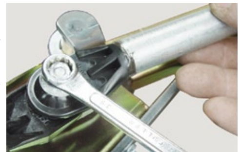
Fig 4: Right - Place the plastic end from the right side cross link onto the top of the first link end on the left side pivot shaft lever. Replace the cup nut on the left side pivot shaft lever.
