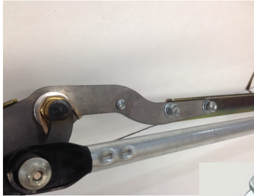
Fig 6: Right - Place the plastic end from the right side cross link onto the top of the first link end on the left side pivot shaft lever. Replace the cup nut on the left side pivot shaft lever.
