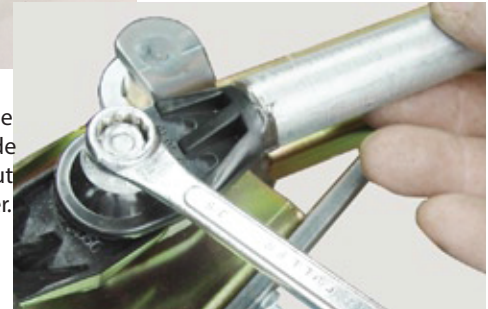
Fig 5: Above - Make sure the right side pivot shaft lever is facing down, similar to the left side pivot shaft lever. The cross link end should be below and slightly to the left of the pivot shaft.
