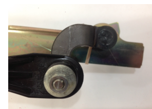
Fig 5: Above - Make sure the right side pivot shaft lever is facing down, similar to the left side pivot shaft lever. The cross link end should be below and slightly to the left of the pivot shaft.
