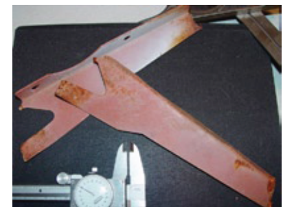
Fig 2: On early F-1s, the two vertical sheetmetal braces beneath the dash panel MUST be removed.
