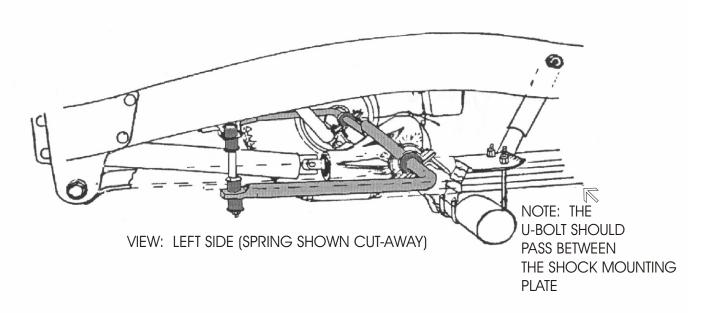
NOTE: ON PASSENGER SIDE OF FRAME, THE FRAME BRACKET MUST BE CENTERED OVER THE RIVET THAT ATTACHES THE SHOCK BRACKET TO THE FRAME.
