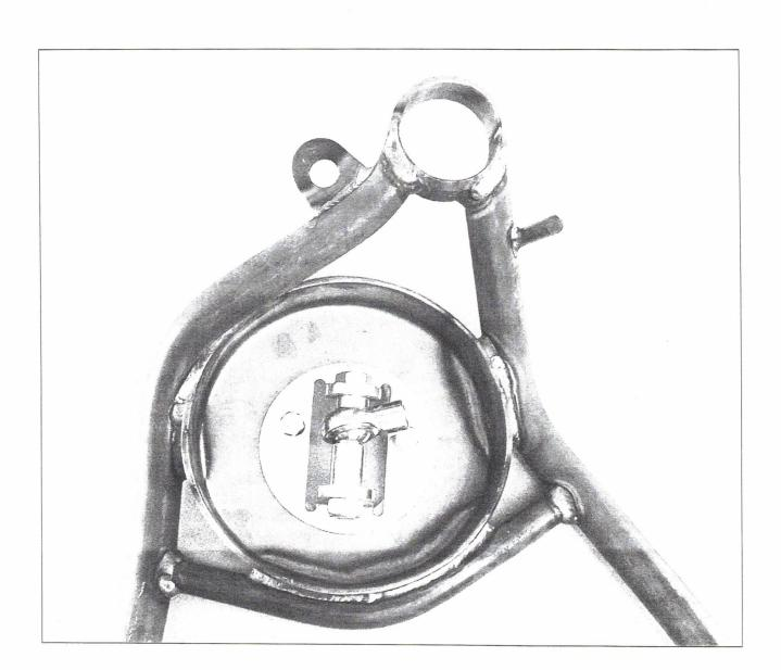
Coilovers will be supplied with a round "foot" with ears to support the lower bearing. That foot is designed to simply bolt into our lower spring cup, without using the urethane seat seen above.
