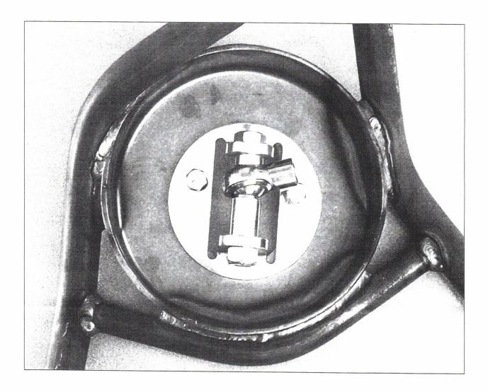
When your arms are ordered to mount an Airride Technologies kit, we supply a ½" thick disc that also bolts into the shock holes in the spring cup welded into the lower arms. They are the
