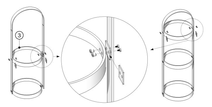
Adjust all the trays at right angles to the handle and tighten the screws.
