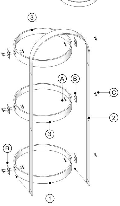
Stick the twin hole pad B to the inside face of the handle 2 so the holes are aligned. Loosely fix the tray with silicon feet 1 to bottom of the handle 2 Before continuing double check you have picked the correct tray for the base.
