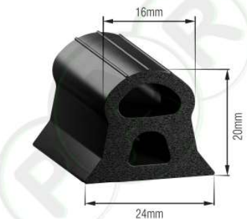
PR325 EPDM/Sponge Universal Double D Seal used on canopies and various lid seals
