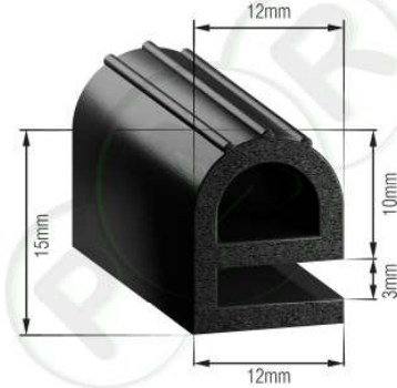
PR316 EPDM/Sponge Universal Small E Seal used on canopies and various lid seals
