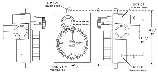
Fig. 3 E-Stop mounting hole locations
