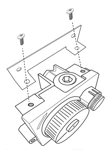
Fig. 1 Installing mounting brackets to ESTOP gas timer.
