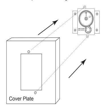
Fig. 5 Installing cover plate.
