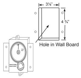
Fig. 3 Installing ESTOP gas timer into wall.
