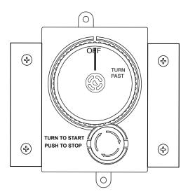
Fig. 4 Shows ESTOP mounted into wall.
