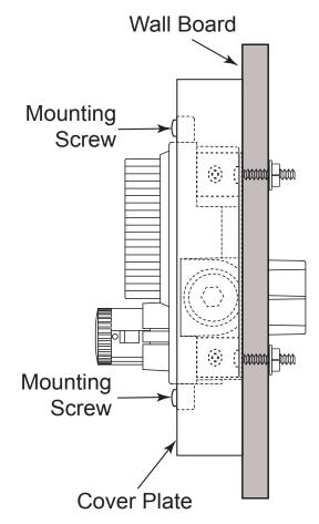
Fig. 6 Side view of ESTOP mounted into wall.
