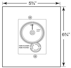
Fig.7 Cover plate outer dimensions.
