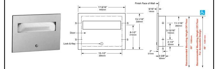
Rough Wall Opening 15-7/8" (405mm) wide 11-7/16" (290mm) high 2-3/4" (70mm) minimum recessed depth
