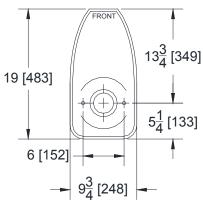
Fixture dimensions meet ASME A112.19.2 / CSA B45.1 requirements.
