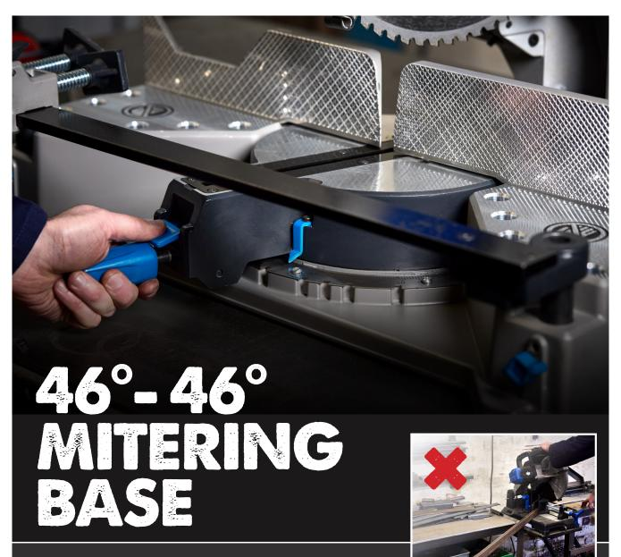
The industry's first 14" chop saw with a mitering base. Enables you to miter your saw instead of the workpiece, so cuts through long materials are quick and easy. Features thumb lock lever and miter detents at common angles for quick, tool free miter setting.
