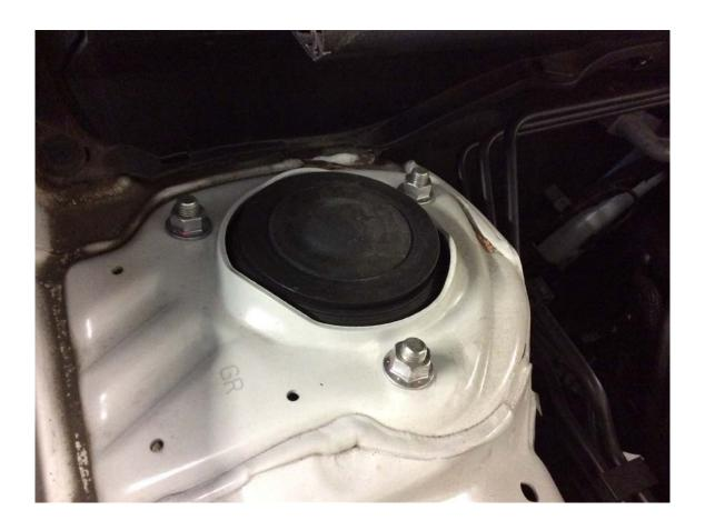
These will be the strut top nuts. Before removing, place a floor jack under the front suspension and take care to make sure the front axle doesn't stretch outwards and pull the CV Joints apart. This may damage the axle and make it unusable, so be prepared in advance even if you hold it towards the car with your knee, etc.
