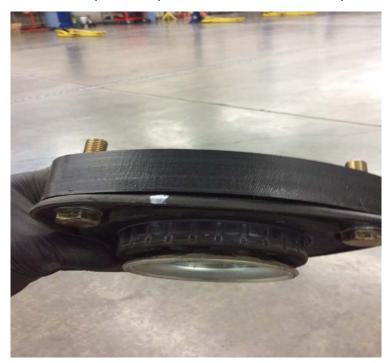
Now you can reassemble the strut, using the alignment marks you placed on the components and spring. The upper nut gets torqued to 41 ft/lbs, then the spring slowly released from the compressor assembly. Once it's completely together and ready to install, make sure the upper portion still rotates smoothly on the upper bearing. To install it's easier to slip the lower portion in next to the axle and then swing the upper portion like this:
