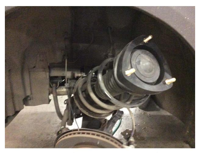
Upper strut nuts get torqued to 15 ft/lbs, and the lower strut bolts are set to 114 ft/lbs after setting the camber bolt position back to your original markings. The alignment will be close, but not exact. Now the wheels can be installed and torqued to the 89 ft/lbs. Before lowering off the jacks and test driving it's a good idea to go back and double check all your nuts/bolts. Better to find an issue parked in a driveway than on the trails or freeway!
