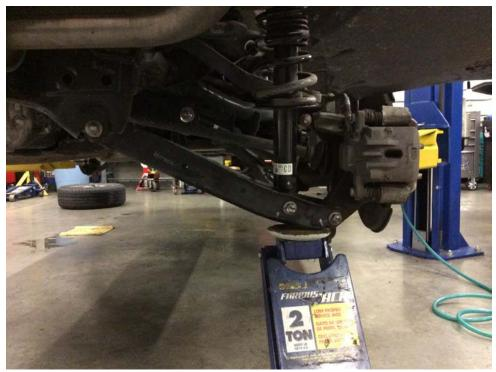
With this bolt removed the link will easily pivot down giving you lots of room to remove the rear strut.
