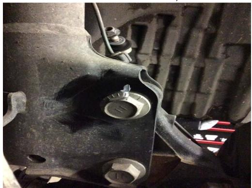
Now remove the 12mm bolt for the brake fluid line on the left and the plastic ABS sensor bracket on the right.
