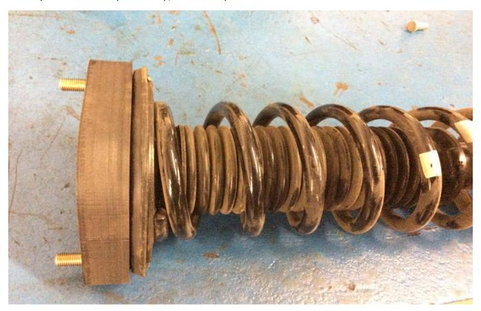
Our kits are computer designed and manufactured to exacting specifications, so if there is any damage or wear to the top of your strut it may take some trying of different angles to get the bolts threaded through the cap and seated. The kits are engineered with brand new strut measurements, but we know they will fit with any correct model year Crosstrek with some effort.
