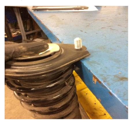
Step 6: Now take one of your spacers with 2 holes and a pair of bolts and washers and assemble as shown below. The washers go between the bolt head and strut cap, and I recommend putting the captured nut in the spacer on top, so that the spacer is held down onto the strut.
