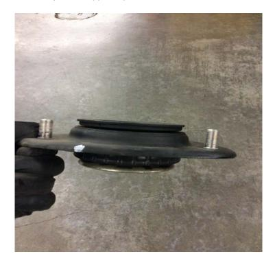
Now you can use the same technique as the rear and with the hammer just remove the 3 studs, install the bolts with washers into the spacer and you're left with a final assembly that should look like this:
