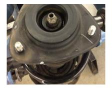
With some tension on the nut it can usually be removed, some may require the rod to be held separately. Once the nut is out, the strut body can be removed through the bottom of the spring and placed aside. The upper portion is where the new studs will be installed. Separate the lower bearing portion and you'll be left with just the upper cap like this:
