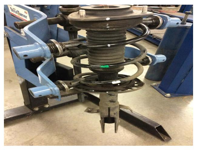
As you can see in the picture, we've marked white reference points on the spring, strut, bearing and upper cap to make reassembly easier. It's not required but helps. Once the spring is partially compressed you can remove the rubber cap on the top to access the strut rod nut.
