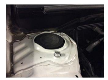
Here again, you can leave one nut on a couple threads to support the weight of the strut to help during removal.
