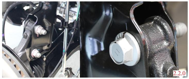
1.9.0 Front Strut Spacer installation. Front Spacers are side specific, spacers will be stamped and marked in white paint pen. (L Driver) & (R Passenger) When installing these the logos should be read looking into the engine bay. Studs market with L and R will be more forwards facing stud. The orientation is extremely important; installing them incorrectly will cause alignment issues and will not go back into spec.
