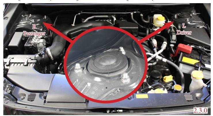
1.10.0 Slide Spacer on correct strut, use factory nuts removed prior and tighten the spacer to the top hat. 14mm End wrench, helps to use the 22mm end wrench to apply pressure to the lift spacer studs to get the lower studs nice and tight. Note: Strut top hat spins, orientation of lift spacer on strut top hat does not matter as they are cimetrical.
