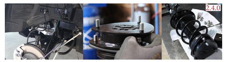
1.11.0 Re install strut with new strut spacer installed. (6) Nuts from Bag "X" (3) per side. Make sure spacer is in correct orientation. 14mm socket to fasten the new spacer and nuts in their location. Torque top hat studs to (22 Ft/Lbs.)
