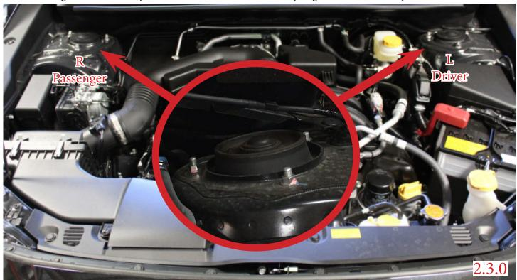
1.10.0 Slide spacer on to the correct strut. Using the factory M12 nuts, tighten the spacer to the top hat. Note: Orientation of lift spacer on strut top hat does not matter as they are symmetrical.
