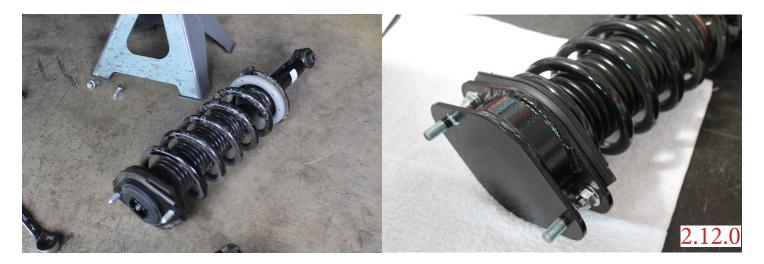
1.33.0 Install rear strut lift spacer on top of strut. These spacers are not side specific. Slide spacer onto strut top hat and use the factory nuts to tighten the bottom of the strut lift to the strut top hat. 14mm end wrench. (Image: 2.12.0)
