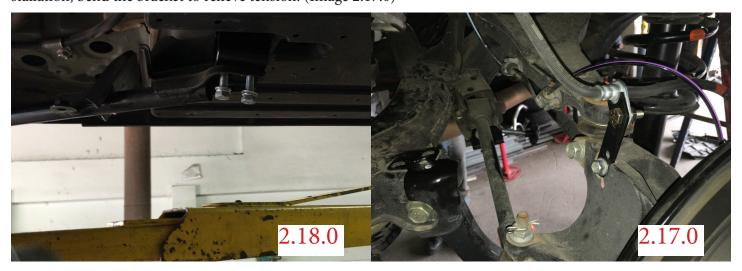
1.46.0 Install forward support arms and spacers. Attach forward support arm to primary support bracket
