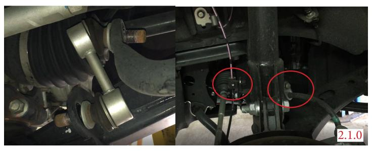
1.9.0 Front Spacers are side specific - stamped and marked in white paint pen (L Driver) & (R Passenger). When installing these, the logos should be read looking into the engine bay from the front of the car (Images 2.1.0/2.5.0). The studs marked with L and R are the furthest forward stud. The orientation is extremely impor-
