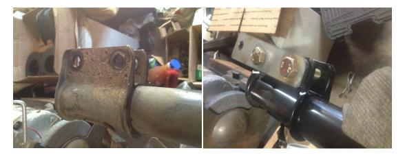
Then you want to use a cut of wheel and cut the lips where you need to cut too. Start to cut from front to the back where you made the notch. Go SLOW! **Take your time and avoid cutting too much and getting the strut to hot**. **Make sure to paint it so it doesn't rust!**
