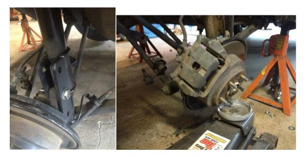
Hardware Fitment: Each new M14 bolt gets one flat washer on the head of the bolt prior to install. There are only 4 nuts in the kit, when placing these they get a washer and a split washer to prevent movement. There only bring 4 nuts in the kit you will use the factory nuts, these are locking flange nuts, they do not need any washers or lock washers when installed.
