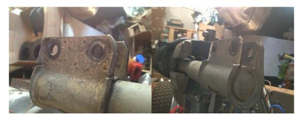
Now that you have them all clean and the plates fit nice and flush with the lower section of the strut (use bolts to make sure it's perfect) begin to install.
