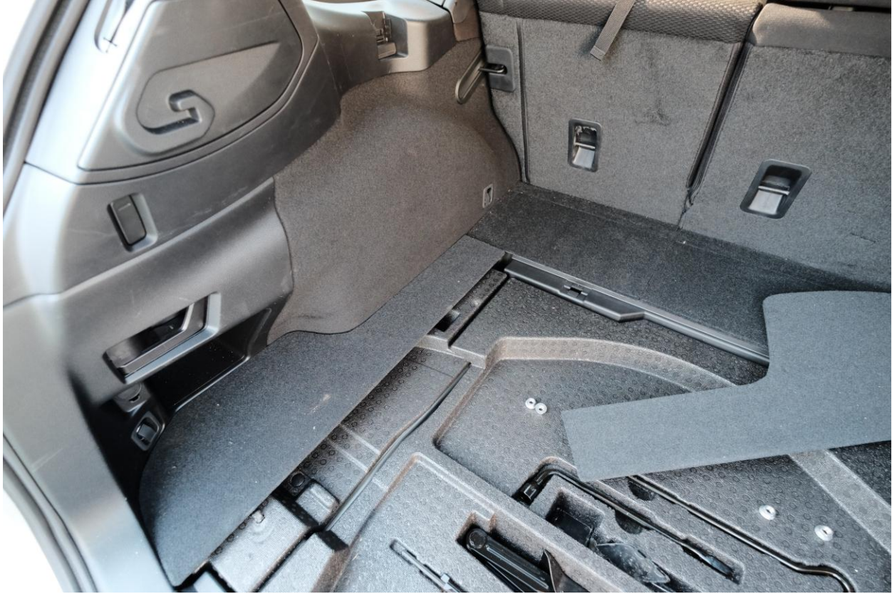
Once all those are removed you will see the two 14mm nuts holding each strut on.
