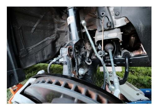
Also of note. DO NOT LET YOUR CONTROL ARM DROP WHEN YOU REMOVE THE STRUT FROM THE KNUCKLE. YOU RUN THE CHANCE OF POPPING YOUR CV JOINT
