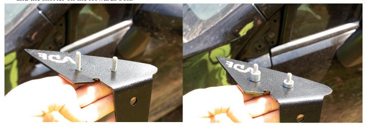
5. Bring the bracket and the hardware up to its mounting location and slowly apply it to its new location. At this point you can finger tighten the rear allen bolt into its hole where we remove the other fender bolt.
