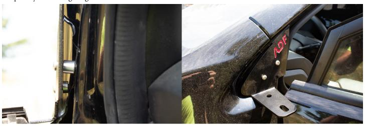
6. Once its finger tight, you will need a 10mm end wrench and some tape. Put a little tape on the back of the wrench and put in the new nut that is provided. You will need to snake this up behind the fender to mount that forwards allen bolt to.
