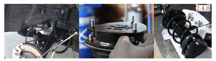
1.11.0 Re install strut with new strut spacer installed. (6) Nuts from Bag "H" (3) per side. Make sure spacer is in correct orientation. 13mm socket to fasten the new spacer and nuts in their location. Torque top hat studs to (14.5 Ft/Lbs.) NOTE: If this is a 1.5" Lift kit with the sapcer that had an acsess hole the ADF logo faces outwards towards the fender. L & R still applies as stated.
