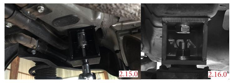
1.35.0 Install all "ADF" Multi link spacers. Bag "#1" (M14 x 50mm) will mount the block to the body. Torque to 106.9Ft/lbs. To torque down these bolts, slide a 3/8" 22mm (7/8") socket into the block, and then run a long 3/8"
