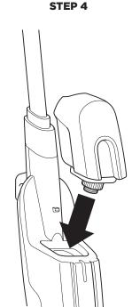
4 To replace the water tank, align it so the cap faces down. Place the cap into the hole in the Steam Mop body and slide tank down until it clicks
