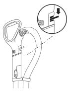
To detach the handle OR from the top of the wand, press the handle release latch.
