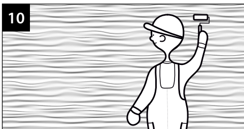
10 Before painting, panels should be primed with WELDPRIMER using a velor roller.
