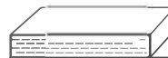
Please note the cutting will expose internal foam structure of the panel. Make sure the cutting edge is at the wall edges and is not exposed.
