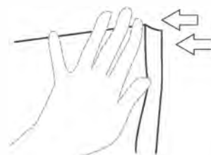
Firmly press the panel and move to the next panel to adjust the edges.
