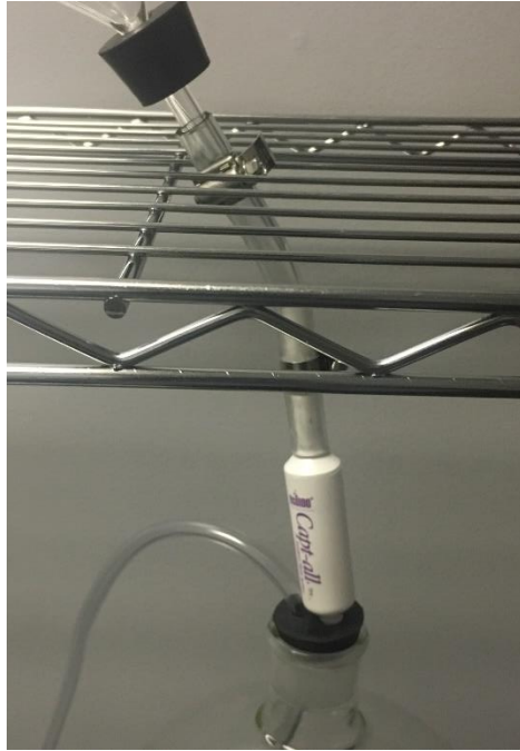
The setup of the Capt-all filter within the apparatus
