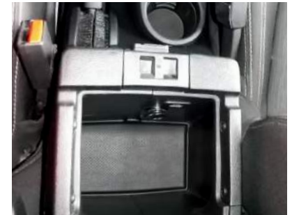
If the vehicle was equipped with Uconnect and the PAC USB adapter is installed, the factory USB port inside the center console will be retained.
