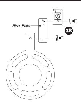
4. Place the completed assembly on the tire carrier wheel studs and install the supplied push nut retainers on the wheel studs.
