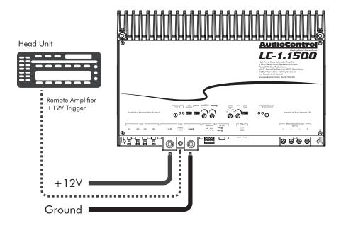
In this example, the head unit has a +12V trigger output that is connected to the LC-1.1500 remote input terminal. When the head unit is turned on, it will turn on the LC-1.1500 amplifier.
