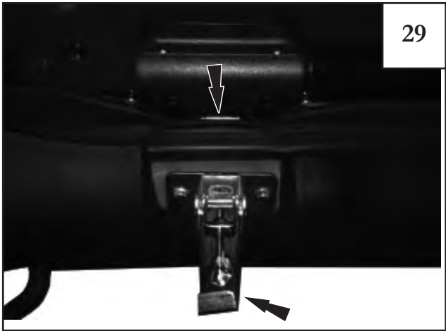
Pull the flip top header assembly tightly against the windshield seal and hook to catch. For proper tight adjustment of the latches, unscrew each front screw hook latch where the latching hook just reaches the header assembly.
