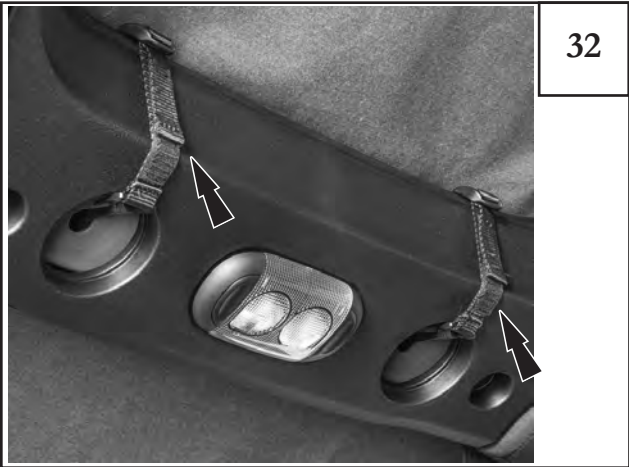
Wrap the two straps attached to the middle section of fabric around the rear-middle of the sound bar.
