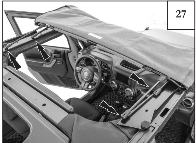
Lift the folded soft top and hardware assembly onto the top of the Wrangler sport bar. Place and center toward the front windshield gasket and line up 4 pivot point clamps as shown.
