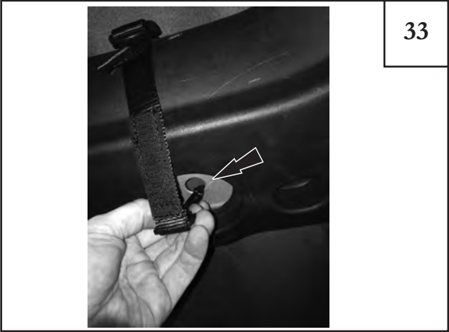
Insert plastic hooks into the holes on the underside of the sound bar. Tighten the strap until snug then hook and loop. TIP: If soft top appear loose on top these can be pulled tighter for tight soft top.
