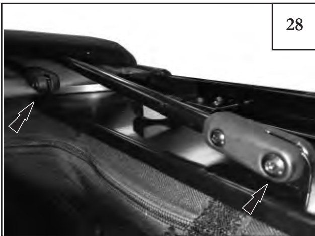
Using the supplied 4mm Allen key, install the Shoulder Bolts from the outside of each soft top header assembly knuckle and tighten each bolt with a lock nut 4 places. The lock nut will fit into plastic.
