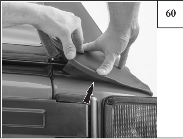
Clip in the last portion of window corner under the rear window retainers as shown.
