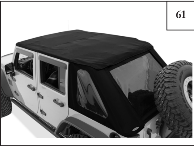
The installation of the soft top is now complete. Be sure all hook and loop flaps are closed.
