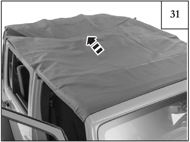
Un-Fold the soft top over the sport bar frame working toward the rear of vehicle.
