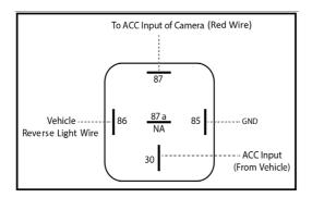
This system is completely signal sensing, there is no "reverse trigger wire" in the wire harness. Some vehicles' reverse lamp wires are now variable voltage wires, and may cause a fuzzy or distorted image. If you experience this, please use a relay to power your camera, as shown in the diagram.
