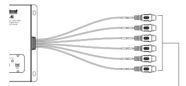
\*\*Pro tip - if using speaker- level/high-level inputs, you'll need some RCA ends on the ends of the speaker wire to attached to the RCA inputs. Setting the Input Level to High of course.
