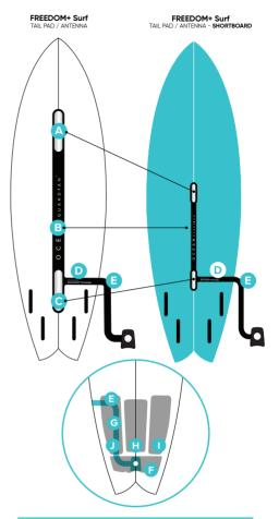
Important note: Please insert the supplied foan Tail Pad Kicker Support when the FREEDOM+ Surf Power Module is not fitted to the kicker.
