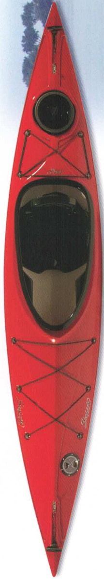
Length: 12 ft. Beam: 26 in. Weight: 41 lbs. Stability: High
