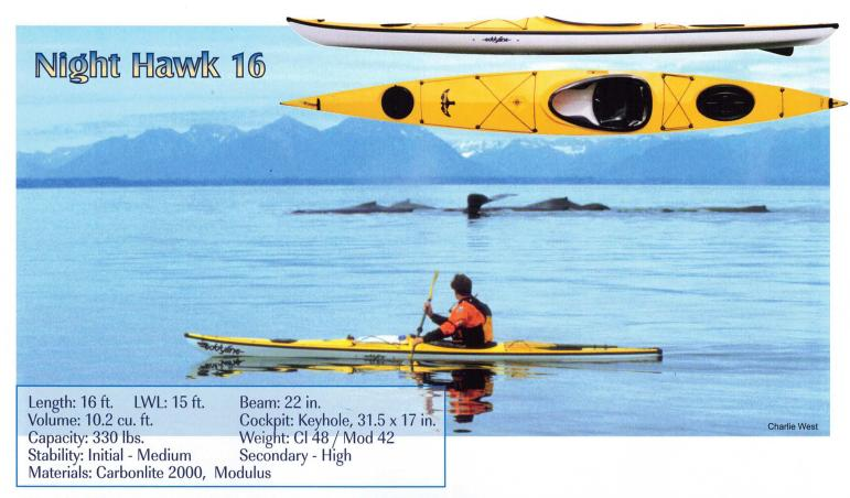
The Night Hawk 16 is a performance kayak with moderate storage capacity. It features a recessed skeg, hatches, bulkheads and a keyhole cockpit along with our comfortable seat and three way adjustable backrest. The Night Hawk 16 uniquely combines speed with high maneuverability and aggressive carving ability. It is quite agile on its own but tracks like a rail with the skeg fully deployed. Even with the skeg, it fits the performance requirements of our designation, Rudder Free Design.
