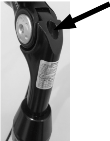
Allen screw 6mm 18-20 N m
