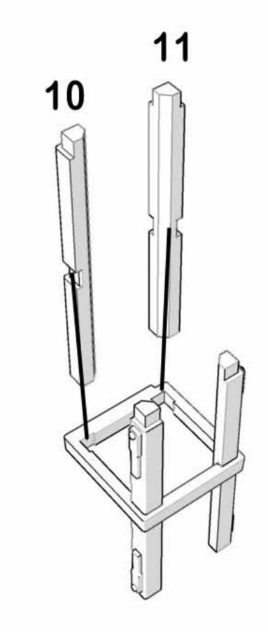
Notes: It is highly suggested that you do not use fast setting glues. Pay special attention when building the cage, noting #8 and where the handles for #12 and #13 align with the notched section for the right and left side launchers.
