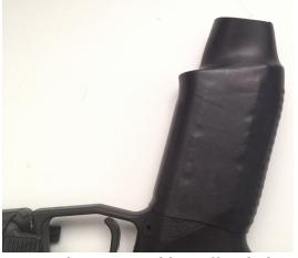
6. Trim the excess rubber off with the razor, flush with the magwell.
