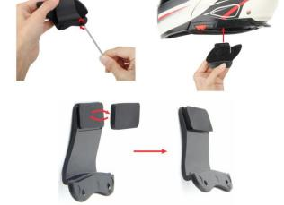
**Note:** Depending on the size and shape of your helmet, you may need to change the thickness of the rubber pad between the clamp plates. You can find two extra rubber pads in the box. To increase the overall thickness, attach the thinner pad to the original rubber pad or replace the original rubber pad with the thicker one.
